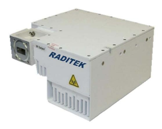
RADITEK's latest 40W and 50W (rated power), Ku band (standard and extended), GaN based BUCs (Block Up Converter) measures only 6.5 x 6.5 x 3.7 inches, and weighs only 5.5Lbs. It is half the weight and 1/3 the size of the closest competitor. It has an very low phase noise LO and a visible LED alarm, in the unlikely event there is a problem.
