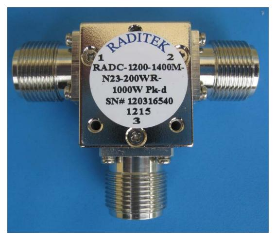
RADITEK's new High Power Coaxial Circulator operates at 1200-1400MHz Full Band. This unit can handle 200 Watts of Average Power and 1 Kilowatt of Peak Power. N-Type Female Connectors are standard and a new compact design of 25.4x28.5x20mm. General Specifications for model shown: Insertion loss (0.35dB), Isolation (20dB min), VSWR(1.25:1).Operating Temperature: -30~+70\*C These units are proven in the field and are fully ROHS compliant.
